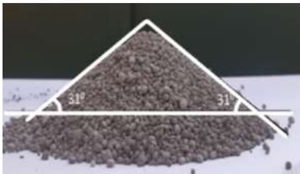
Figure 3. Example of a scheme for measuring the static natural slope angle of superphosphate mineral fertilizer.
