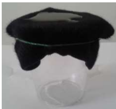
1-rasm. Poliakril gazlamasini suv shimilishini aniqlash.
