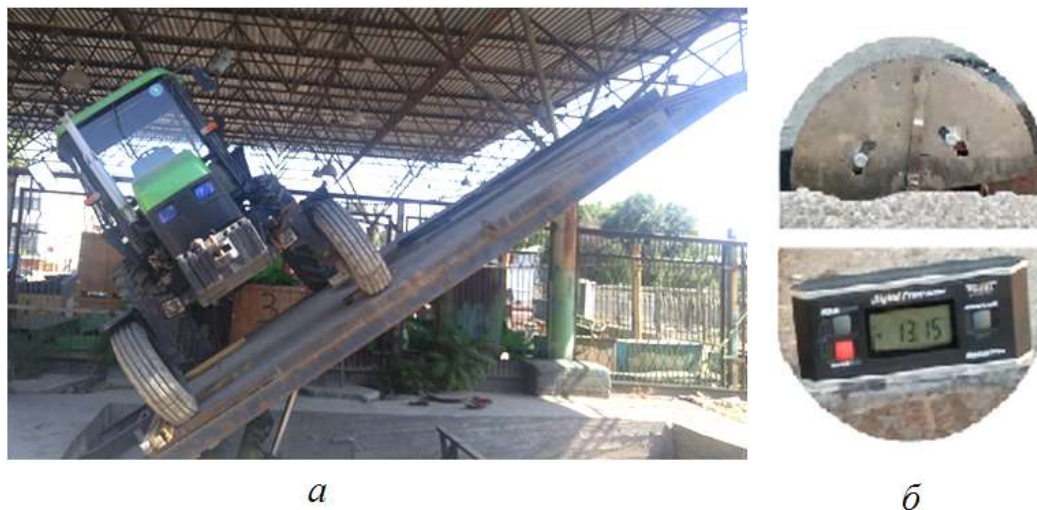
Fig.2. Stand for testing the tractor for lateral stability.
